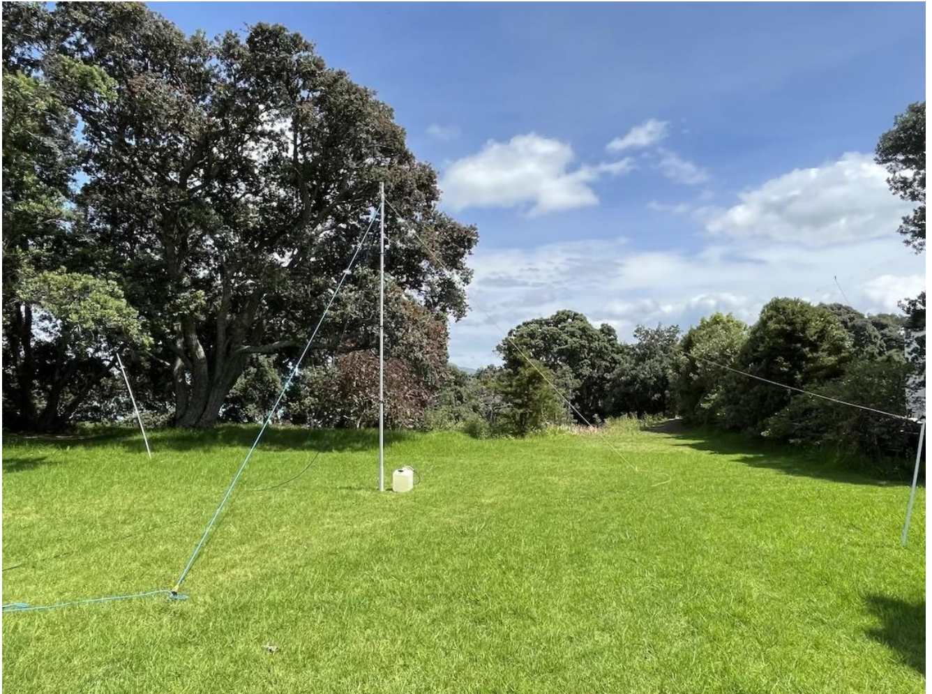
Merv ZL1SK's portable extendable 5 meter pole set up with portable 40 meter dipole.
